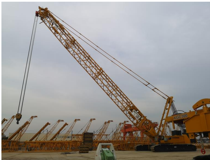
Fig. 1. the crawler crane
