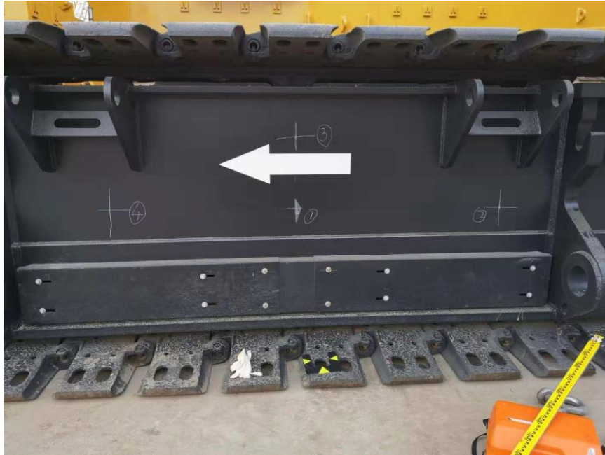
Fig. 2. Determining the measuring points of the crawler crane
